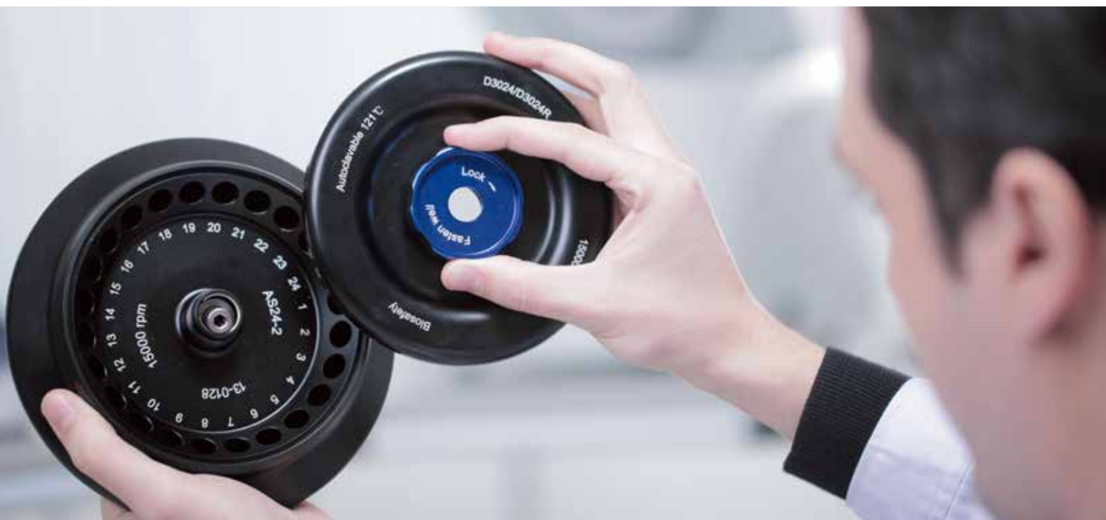
Seals within the aluminum alloy rotor
